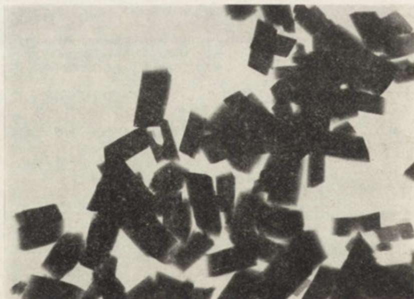
Fig. 3. Electron micrograph of Ca-NHA precipitate. Uniform, cuboidal crystals were formed in test tube by mixing of 0.1 mM \text{CaCl}_2 with 5 mM NHA. Magnification — 20 000 \times
