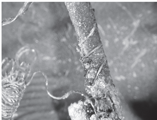
Fig. 4. Microscope picture of a stem made of twisted wire wrapped around with paper, being a constructive element of artificial flowers and served for fixing glass beads. Photo by M. Nowak
