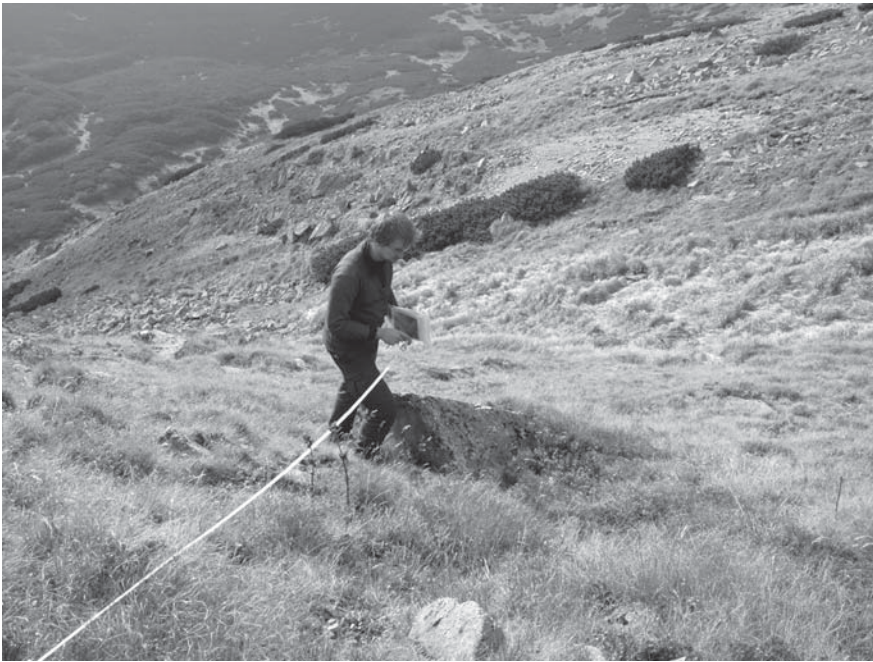
Figure 7. Measuring ploughing boulder (site no. 10) displacement on the SW slope of Mt. Brestová.
