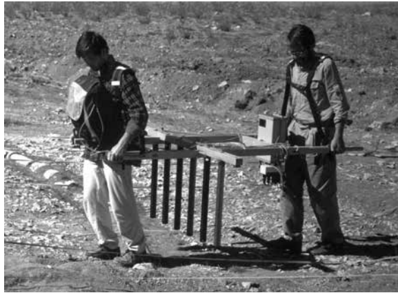
Fig. 27. Harald Stümpel (right) and Ercan Erkul of the Univeristy of Kiel surveying the Hittite site of Sarissa in Anatolia, Turkey, with a system of five fluxgate sensors mounted on a portable rack. Archive of H. Stümpel
