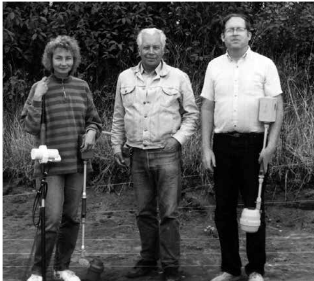
Fig. 23. From left to right: Tatyana Smekalova with an Overhauser magnetometer GSM-19WG by GEM Systems (Canada) and cesium magnetometer M-33 by Geologorazvedka (Russia), Olfert Voss and Bruce W. Bevan with MMP-60 proton magnetometer by Geologorazvedka on the iron smelting site of Snorup in Jutland, Denmark, in 1996. After Smekalova et al. 2005: 16
