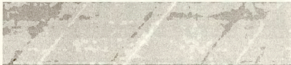
FIG. 6. Regions of plastic deformations created during martensite transformation caused by deformation of TiNi shape memory alloy in temperature 333 K.
