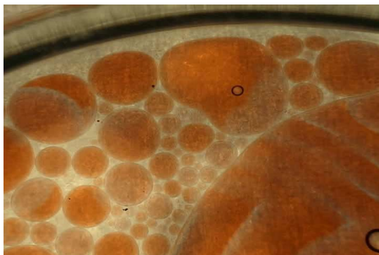
Figure 5.1: BZ droplets immersed in 5 mg/ml asolectin solution in a Petri dish. The thickness of the dish wall is 1 mm. The standard BZ solution composition: 0.3 M sulphuric acid, 0.45 M bromate, 0.35 M malonic acid, 0.06 M bromide, 1.7 \times 10^{-3} M ferroin (video 1 on the accompanying CD).
