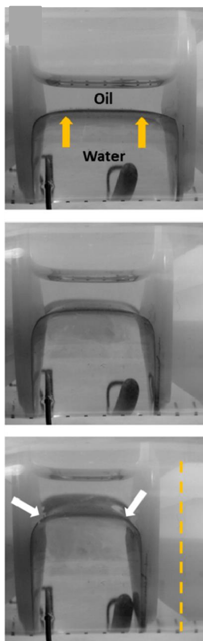
Fig. 49. Demonstration of mechanical properties of the AuNP monolayer. Subsequent stages of the deformations of the film located at the oil–water interface. The yellow dashed line represents the initial position of the mobile piston. When the mean curvature attained a critical value, the film cracked in two places indicated by the white arrows. The yellow arrows indicate their initial positions. The outer diameter of the cylinder is 3 cm.
