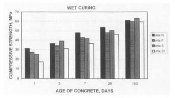
FIGURE 4. Development of cube strength of SLWAC (structural lightweight aggregate concrete) – wet curing.
