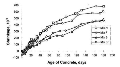
FIGURE 12. Effect of cement replacement materials on the drying shrinkage of SLWAC.
