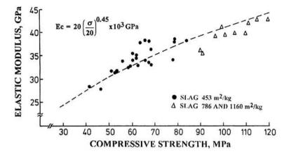
FIGURE 3. Strength-elastic modulus relationship of PC-SLAG concrete.
