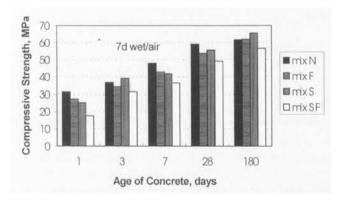
FIGURE 5. Development of cube strength of SLWAC under air drying.
