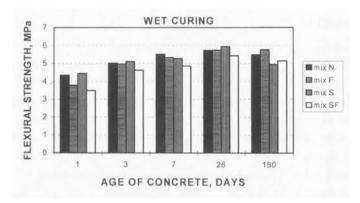
FIGURE 6. Development of flexural strength of SLWAC under wet curing.
