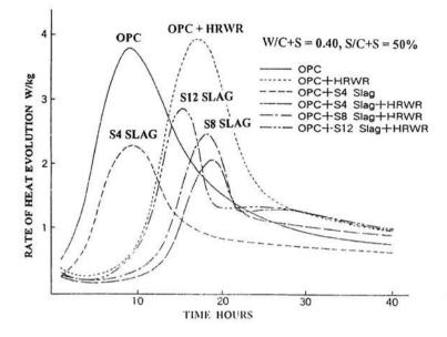
FIGURE 1. Heat of hydration of PC-SLAG-HRWR system.
