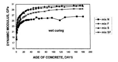
FIGURE 8. Dynamic modulus of SLWAC under wet curing.
