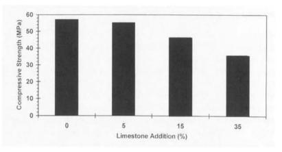
FIGURE 14. 28 day compressive strength of PLC mortar [64].
