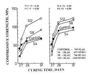
FIGURE 2. Strength development of PC-SLAG concrete.
