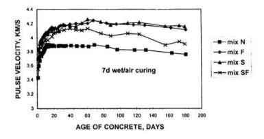
FIGURE 11. Pulse velocity of SLWAC under air drying.
