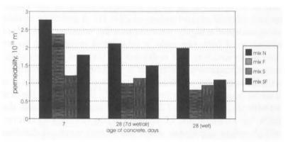
FIGURE 13. Oxygen permeability of SLWAC.
