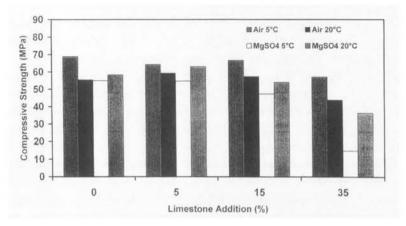
FIGURE 15. One year compressive strength of PLC mortar [64].
