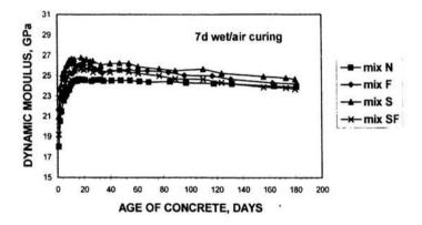
FIGURE 9. Dynamic modulus of SLWAC under air drying.
