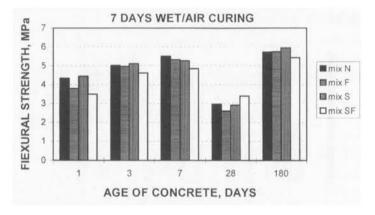
FIGURE 7. Development of flexural strength of SLWAC under air drying.
