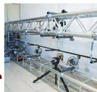
Fig. 4.4.7. Control of structures subjected to traveling loads
