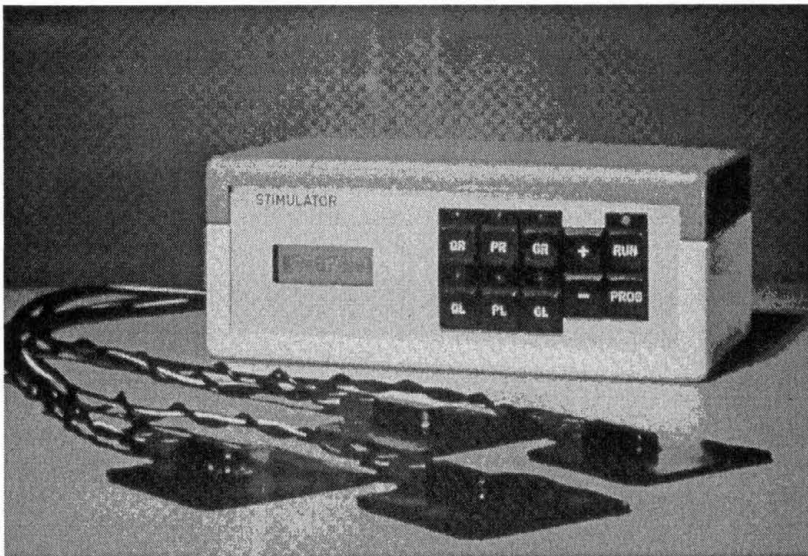
FIGURE 2.3. A six-channel lightweight, portable and computer-controlled stimulator for the functional activation of paraplegic patients [Isakov et al., 1993; Minzly et al., 1993b]
