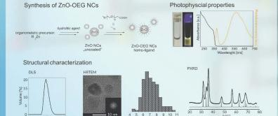
Size distribution of ZnO-OEG NCs in water estimated by DLS; HRTEM micrographs statistical analysis of the size of ZnO-OEG NCs (mean size:  $7.1 \pm 1.1$  mm); the PXRD profile of ZnO-OEG NCs (black line) and simulated ZnO pattern (gray line). Based on the reflection broadening, according to the Scherrer equation, the crystallite size has been estimated to be  $6.0 \pm 0.2$  mm.
