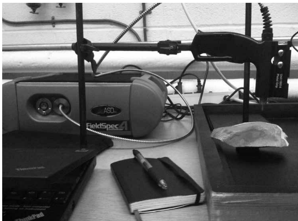
Fig. 3. An ASD Inc. FieldSpec® spectrometer used to obtain spectra in the visible and near-infrared regions. Photo: R.M. Parish.
