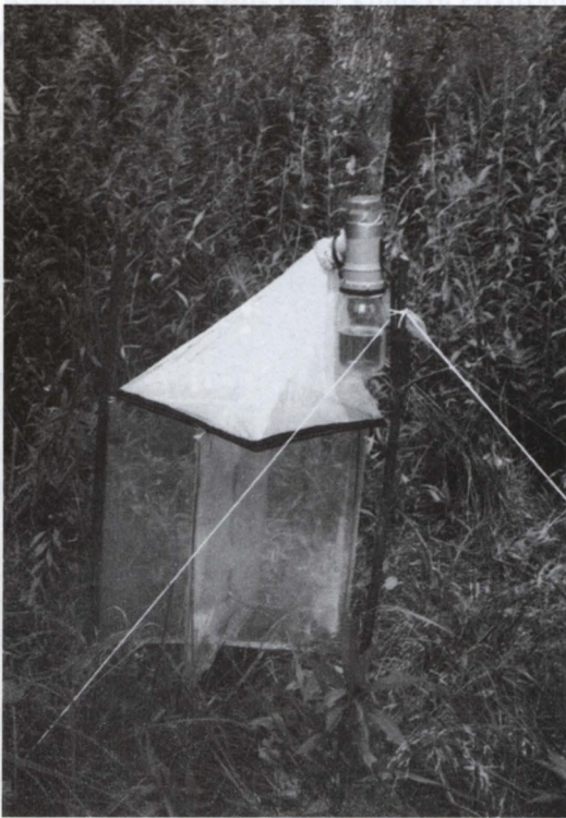
Fig. 5. A screen-Malaise trap instaled in an alder swamp in the range Ameryka (Forest District Berówka)
