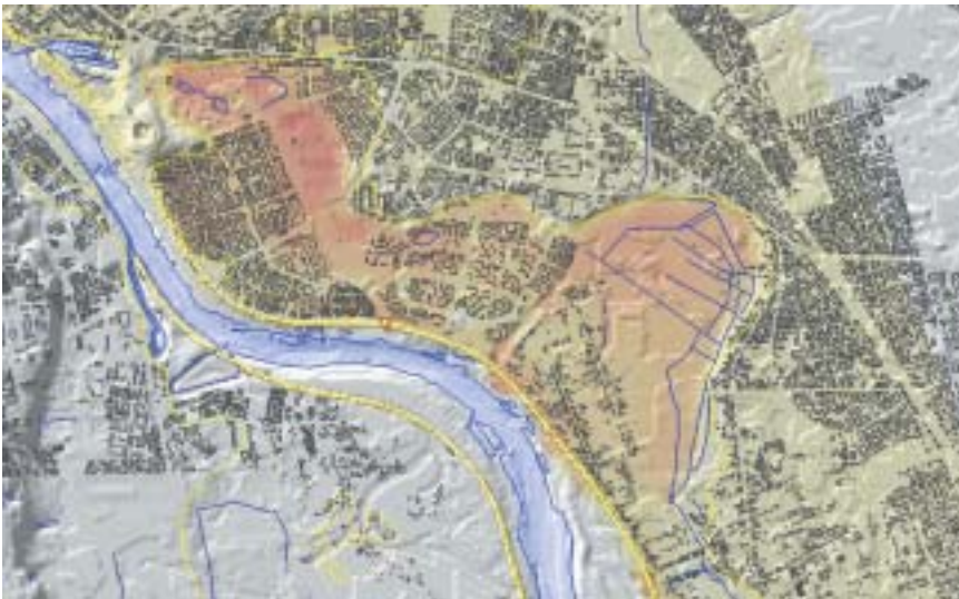
Figure 2b. Range of potential flooding due to dike breach by Q_p 1% at Saska Kępa after 12 h., colours represent depth of inundation, line shows range of inundation obtained from 1D model.
