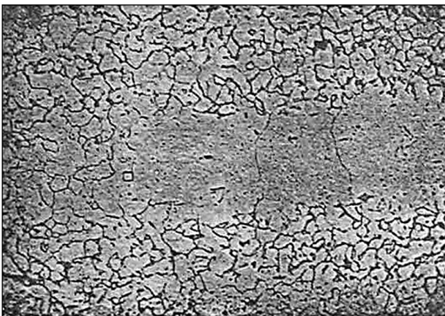
Fig. 2. Microstructure of the blade of the sword from Gdańsk, the Castle Museum in Malbork, Dep. 76. Sample was etched with nital, 100x. After J. Piaskowski 1959, 170, Fig. 116.
