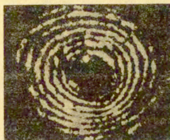
Fig.15. Interference pattern of ultrasonic transducers obtained by holographic method
