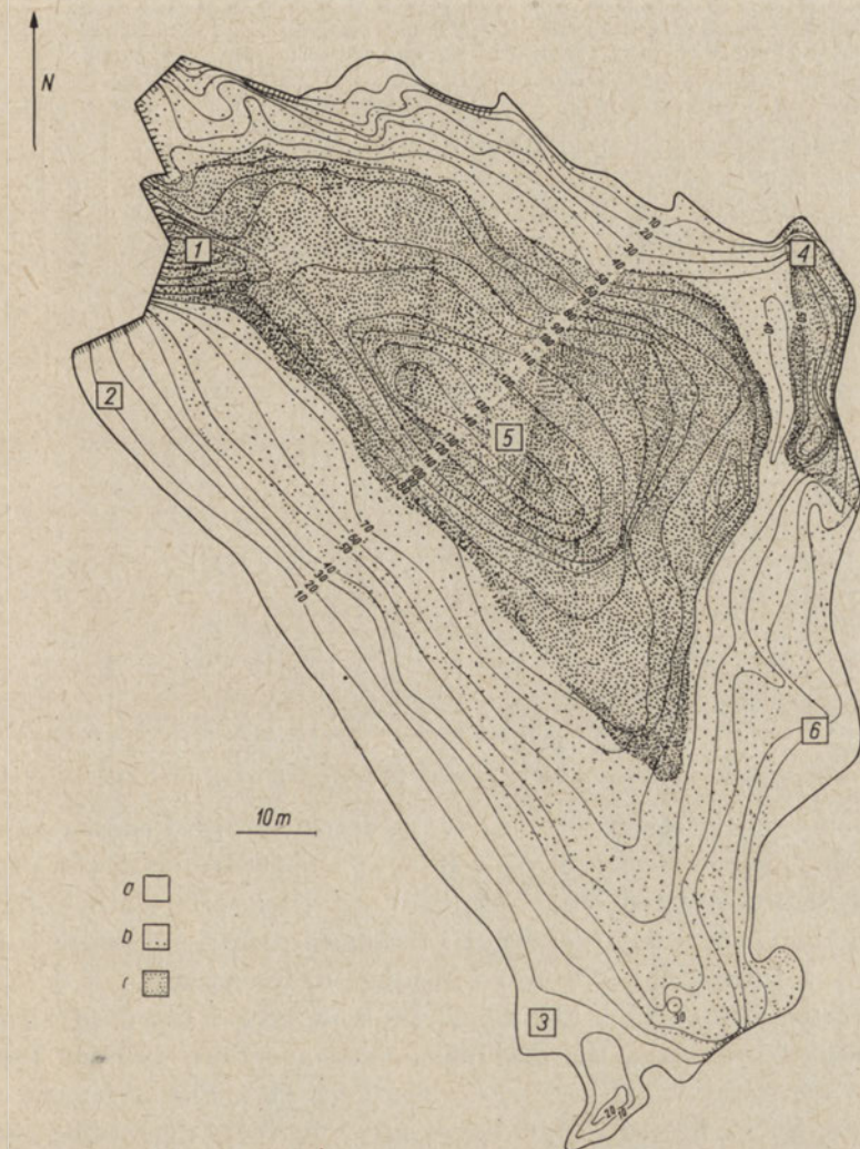
Fig. 2. Izobates of the rocky floor and zones of bottom distinguished in the Duck Pond a — stones, b — detritus between stones, c — detritus covering stony floor, 1—6 — points where thermal measurements were taken
