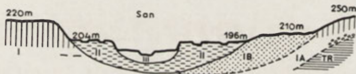
Fig. 7. Section across San valley, from Walawa to Starzawa, after A. Łomnicki [42] III — meadow terrace, II — rendzina terrace, I — Diluvial terrace, IB — Diluvial sands, IA — Diluvial clays, TR — Tertiary (Krakowic clays).
