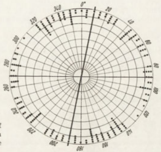
Fig. 24. Diagram of the arrangement of pebbles in a fluted moraine 1–1.5 m from the morphological axis of the ridge
