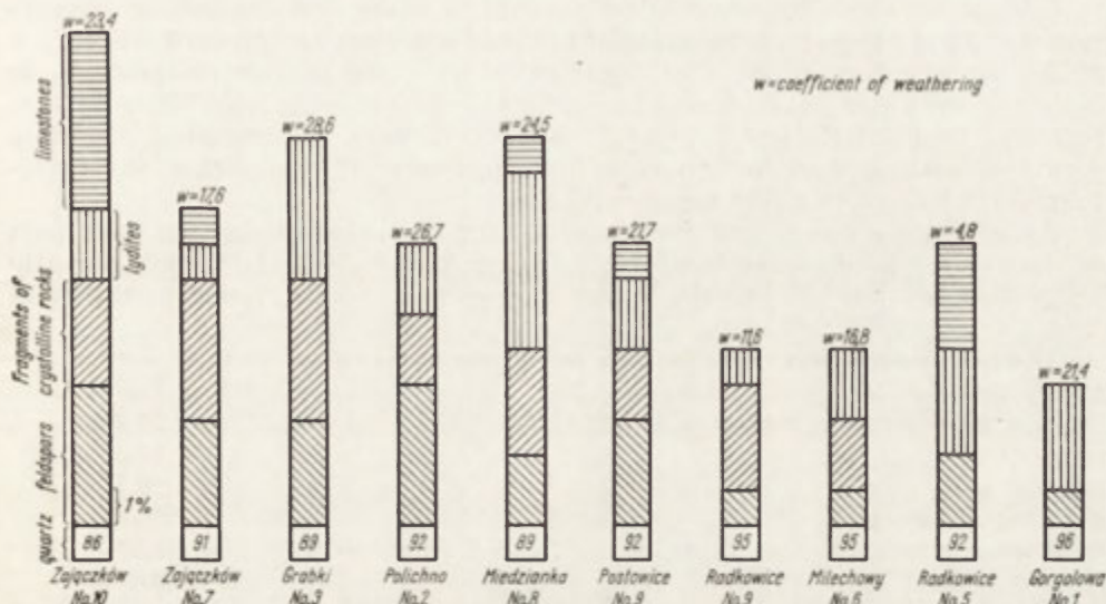
Fig. 22. Petrographic composition of sands on basis of an analysis of the 0.5–0.8 mm fractions
