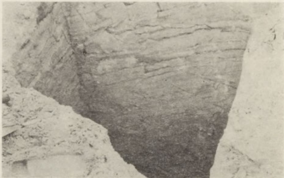
Photo 1. Polichno — a test pit in a kame terrace in a mountain pass. The parallel stratification of fine grained sand deposits (fine grained medium sand as defined by Doeglas, 1968) can be seen
