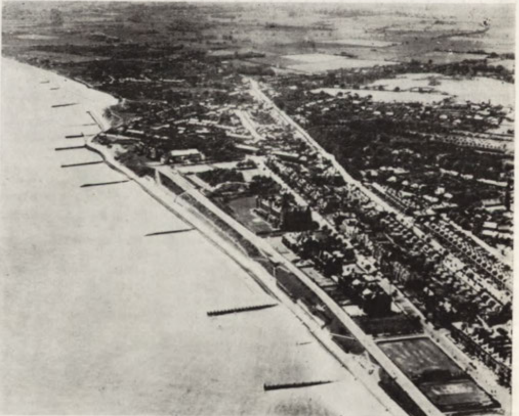
Fig. 10. Lowestoft Harbour, England: an example of terminal scour due to the construction of walls and groynes (after Aerofilms)
