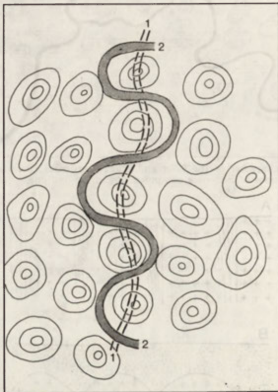
Fig. 12. Formation of meanders (structure controlled meanders) of the Bóbr River by adapting of the river to subsurface knobs of granite bed-rock 1—initial stage of river on the surface of weathering products, 2—stage of river after skeletonizing hard knobs of bed-rock
