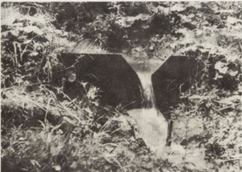
Photo 4. Sharp-crested triangular weir for measurements of concentrated overland flow
