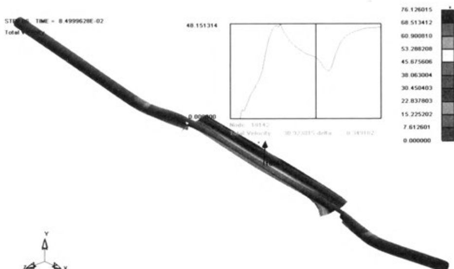
FIGURE 3. Numerical values of the parameters of a large piece of debris produced under rupture of underground main gas pipeline (a scale of the von Mises equivalent stresses [MPa], a plot of velocities [m/s]).
