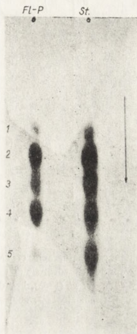
Fig. 13. Identification of sugars of the flavoprotein by chromatography on Whatman no. 1 paper with n -butanol - pyridine - water (5:3:2, by vol.). The spots were located with the aniline-phthalate reagent. FL-P , flavoprotein hydrolysate; St. , standards: 1, glucosamine; 2, galactose; 3, glucose; 4, mannose; 5, fucose.
