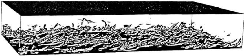
FIGURE 6. Coherent structures of a turbulent flow at Re_\tau = 100 , after Temam et al. [184]
