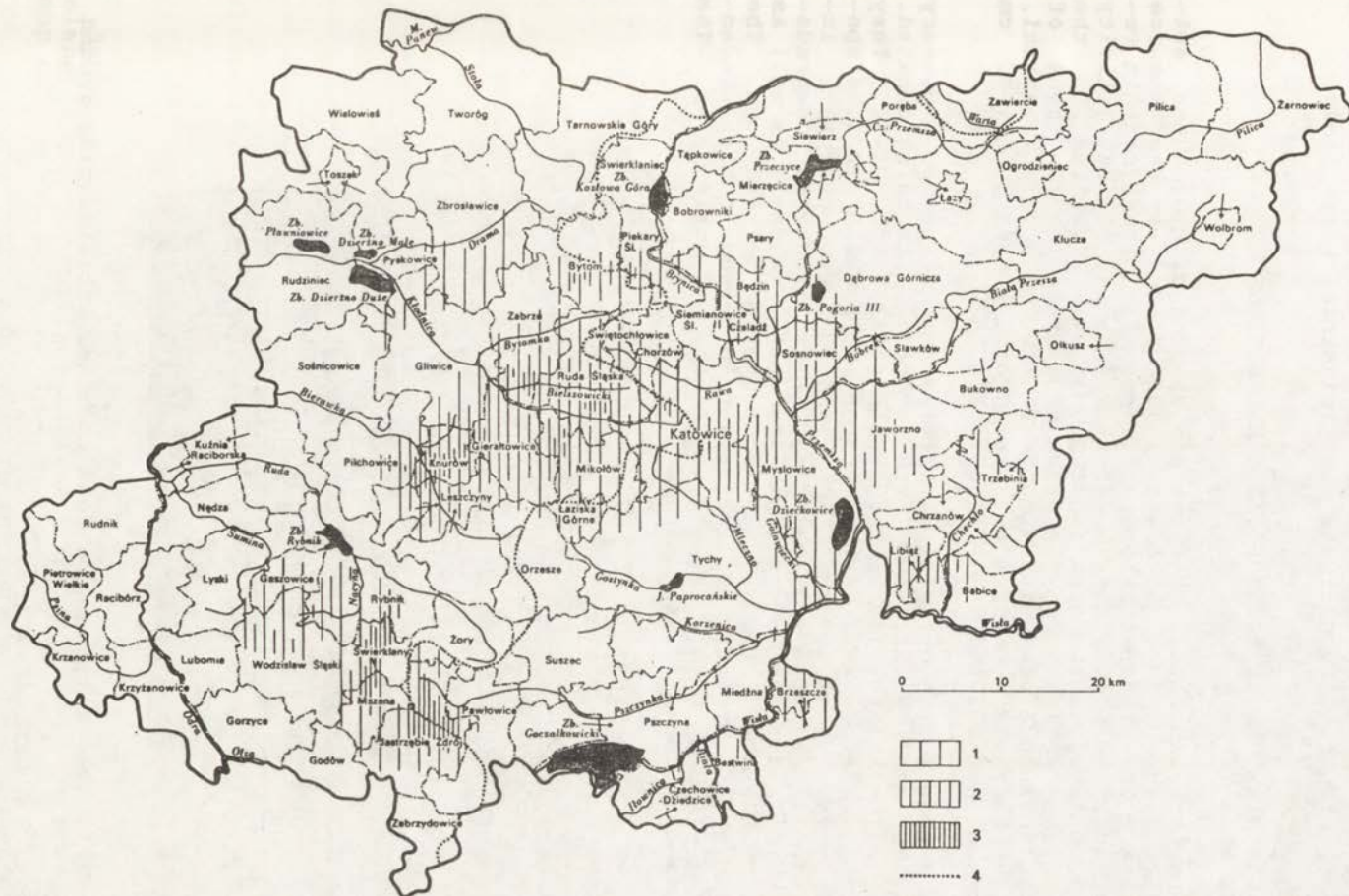
Fig.4 Zones of ground subsidence in Katowice province: 1—from 0 to 5 m, 2—from 5 to 15 m, 3—more than 15 m, 4—watershed dividing the Odra and the Vistula drainage areas
