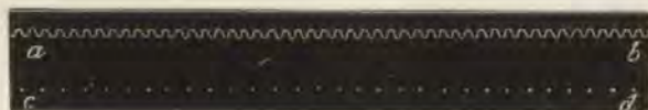
FIG. 30.—GRAPHIC REPRESENTATION OF RATE OF VIBRATION OF BEE'S WING. a, b , Line Made by Tuning Fork; c, d , Marks Made by Vibrating Wing.
