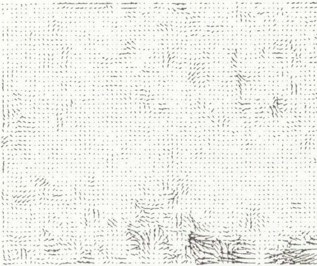
Fig. 3b Instantaneous slip velocity field, i.e. velocity field of fluorescing particles less the velocity field of tracer particles. The vector scale in Fig. 3b is twice that in Fig. 3a.
