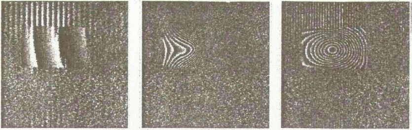
Figure 3: Compensation of motion components by subtraction of linearly varying phases
