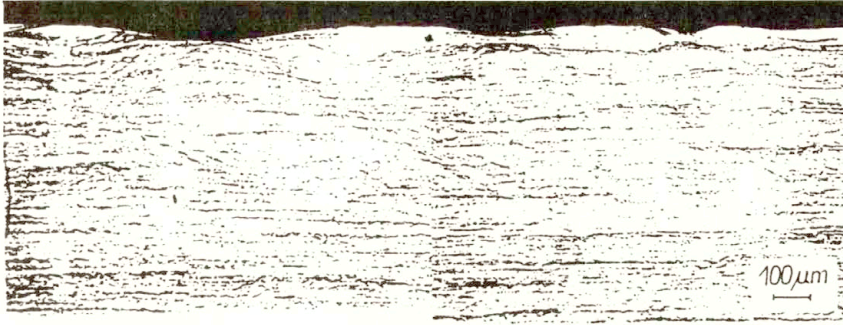
FIG. 2. Transcrystalline propagation of the shear bands (seen within the neck) through many grains in stainless steel [24].
