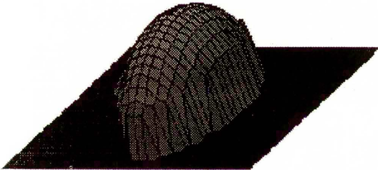
FIG. 2. Opening of a crack of elliptical form. The semi-axes ratio 2 : 1.
