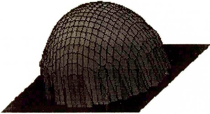
FIG. 1. Opening of a crack of elliptical form. The semi-axes ratio 1 : 1.
