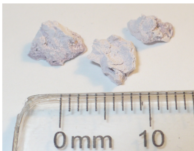
Figure 59: The picture of as prepared solid silica mesophase doped with Au NPs. Slightly violet color of obtained material, results from the presence of gold NPs.
