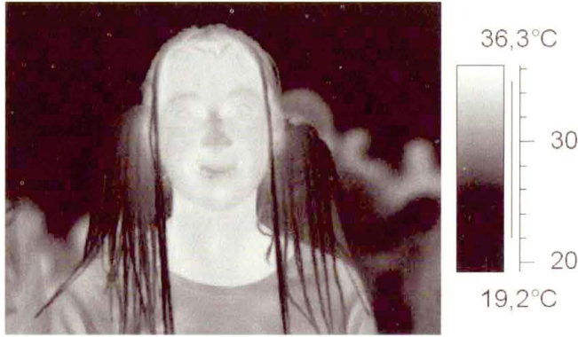
FIGURE 14. Emitted infra-red radiation can be captured and used to visualize surface temperature.
