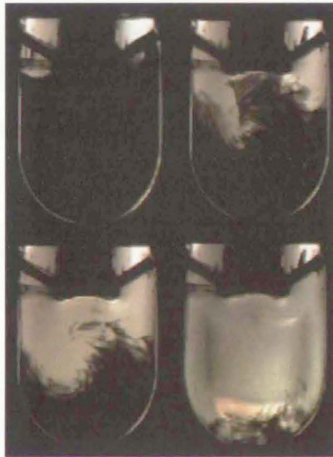
FIGURE 32. The paint erosion method permits the visualization of the distribution of wall shear stress.
