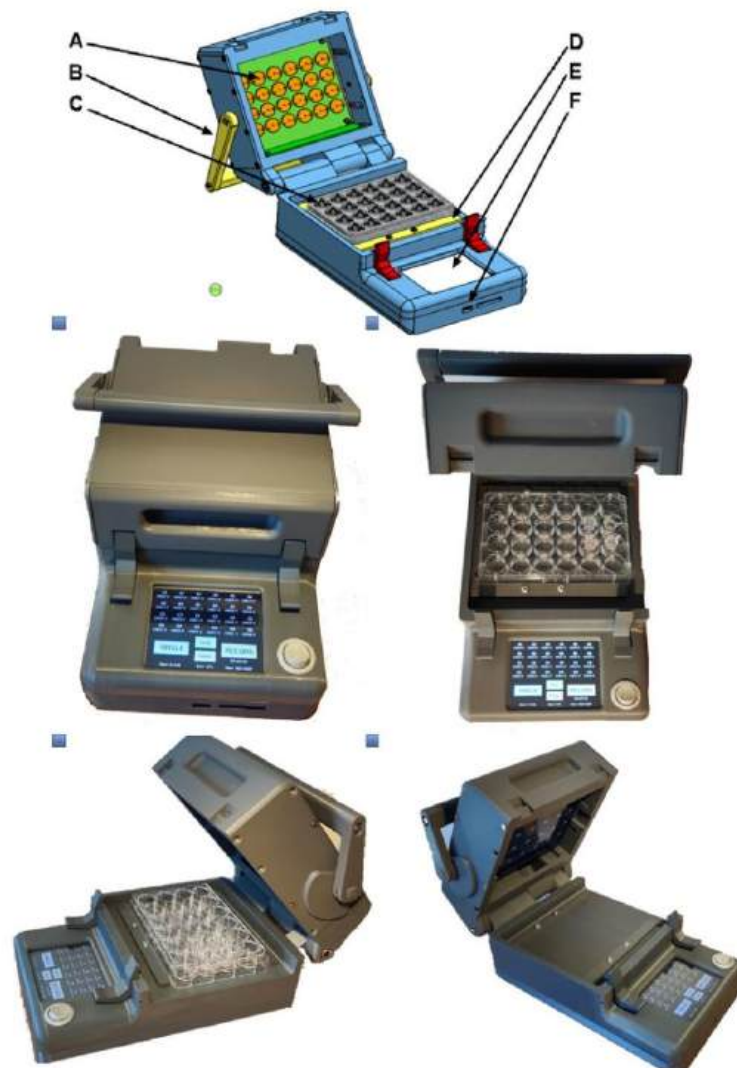
Fig. 3. Construction of MS with culture plate guide; A. head with electrodes. B. lowering lever. C. cell culture plate, D. position adjustment of cell culture plate, E. LCD, F. memory card input.
