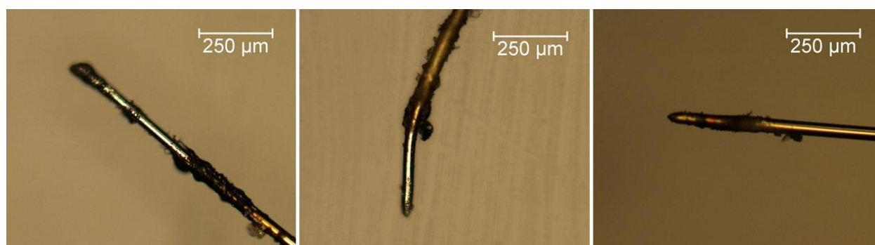
Fig.12 Microscope images of insulation damage of different 25µm electrodes (laser parameters used; power 80%, and speed 80.0).
