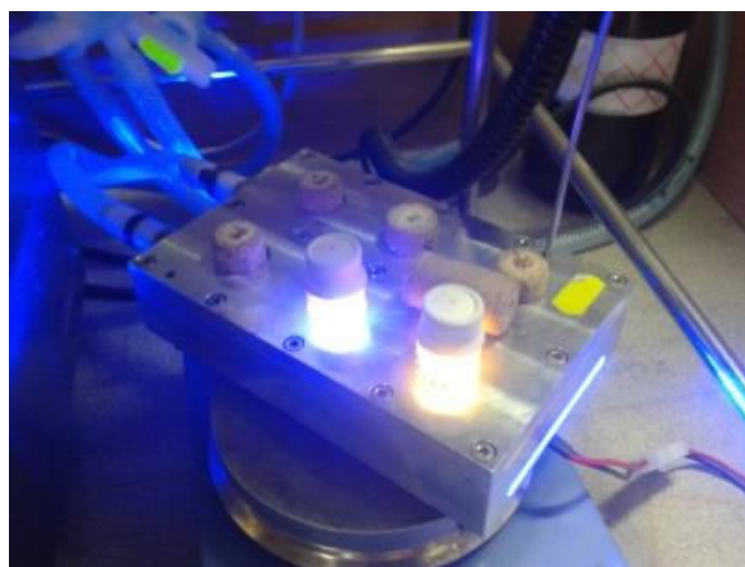
Figure S1. Photoreactor setup with aluminum cooling block
