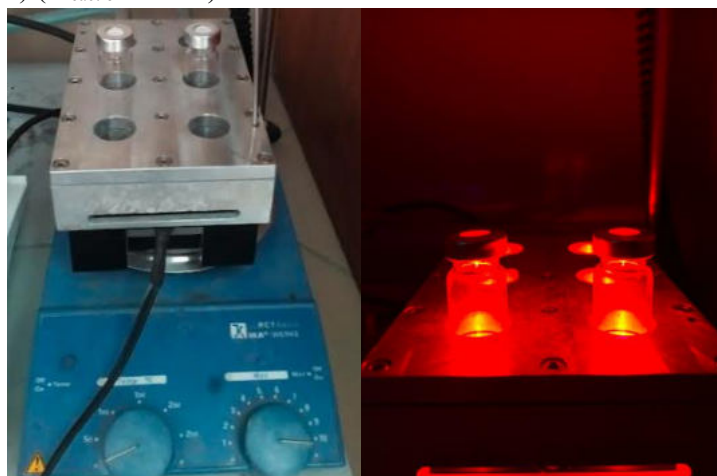
Figure F2. Standard photoreactor setup (660 nm, 3 W).
