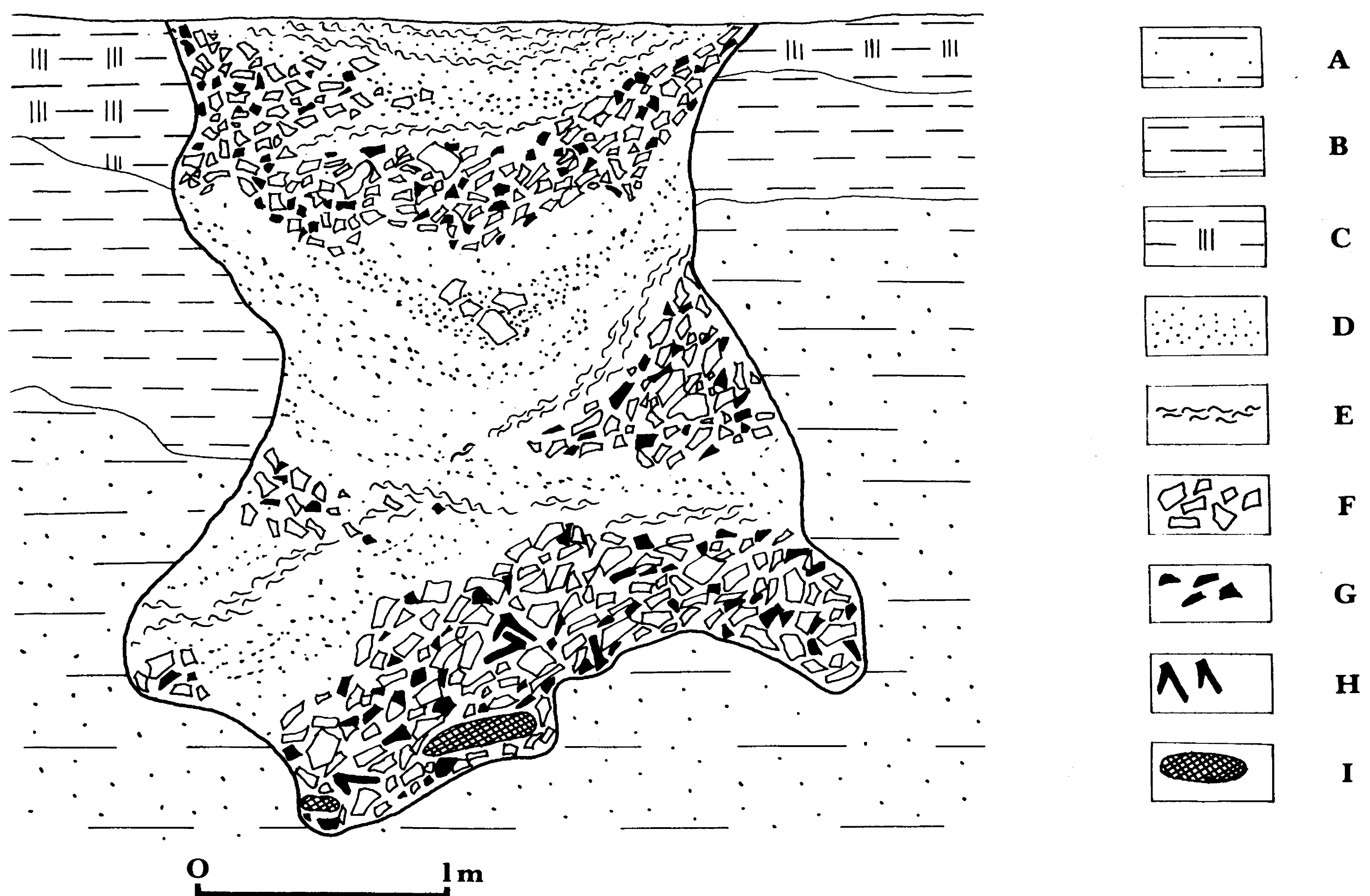
Fig. 2. CZ 1 Tušimice, Chomutov dist. Section of the shaft no. 5: a — mother sandstone with quartzite nodules; b — grey, brown and yellow clays; c — black silt; d — clays in secondary position in filling of the shaft; e — silt in secondary position in filling of the shaft; f — sandstone rubble; g — quartzite industrial waste; h — antler picks; i — hearths. After E. Neustupný.
