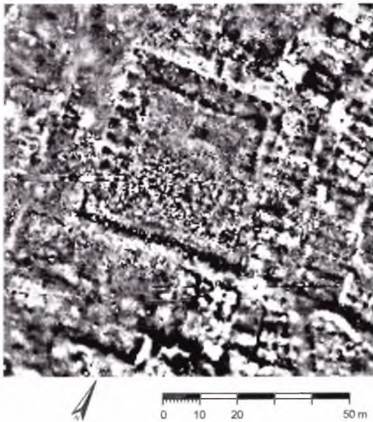
Fig. 2. Kharab Sayyar, Raqqa District, Northeast Syria. Magnetometer survey 2000–2002 (fluxgate gradiometer Förster Ferex 4.032 DLG, four channels, base distance 0.65 m, 0.25/0.5 m inline/crossline). 256-greyscale-plot with mosque and part of the suq (dynamics: -4/+4 nT black/white).
