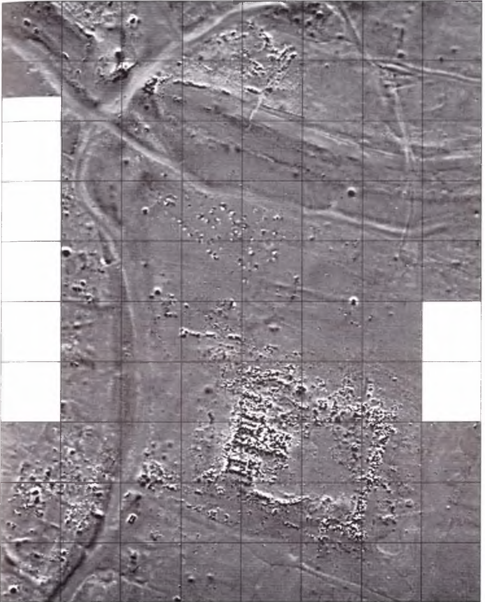
Fig. 1. Uruk. Magnetogram of the southwestern part of the city. Magnetogram in grey shading with 256 greyscale. Caesium magnetometer Smartmag SMG4-Special in duo-sensor configuration, dynamics \pm 10 nT (white to black), sensitivity \pm 10 pico-Tesla, raster 0.5/0.1 m interpolated to 0.25/0.25 m, dynamics of the total magnetic field 45230 \pm 30000 nT, line mean over 40 m, desloping and edge matching, 40 m grid, north to the top.
