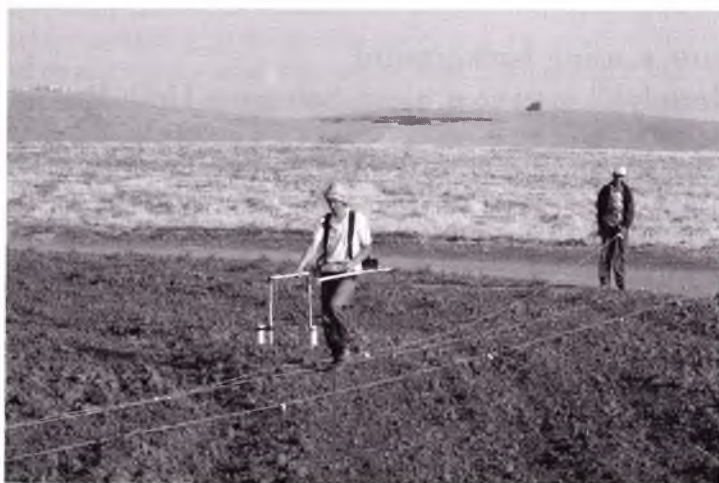
Fig. 1. Tell Mozan. Modified caesium magnetometer G 858 in the lower city.
