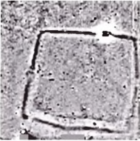
Fig. 1. Iron Age enclosure system surveyed with a dual FM 256 system (FM 256 master + FM 36 slave). Grey scale range \pm 3 nT. Data was sampled at 0.7 s/m, 4 readings/m, traverse interval 1 m, zig-zag mode. Processing interpolates this to sample and traverse intervals of 4/m. Area = 1 ha, survey time just over 2 hours. Data shown courtesy of the Huddersfield and District Archaeological Society.
