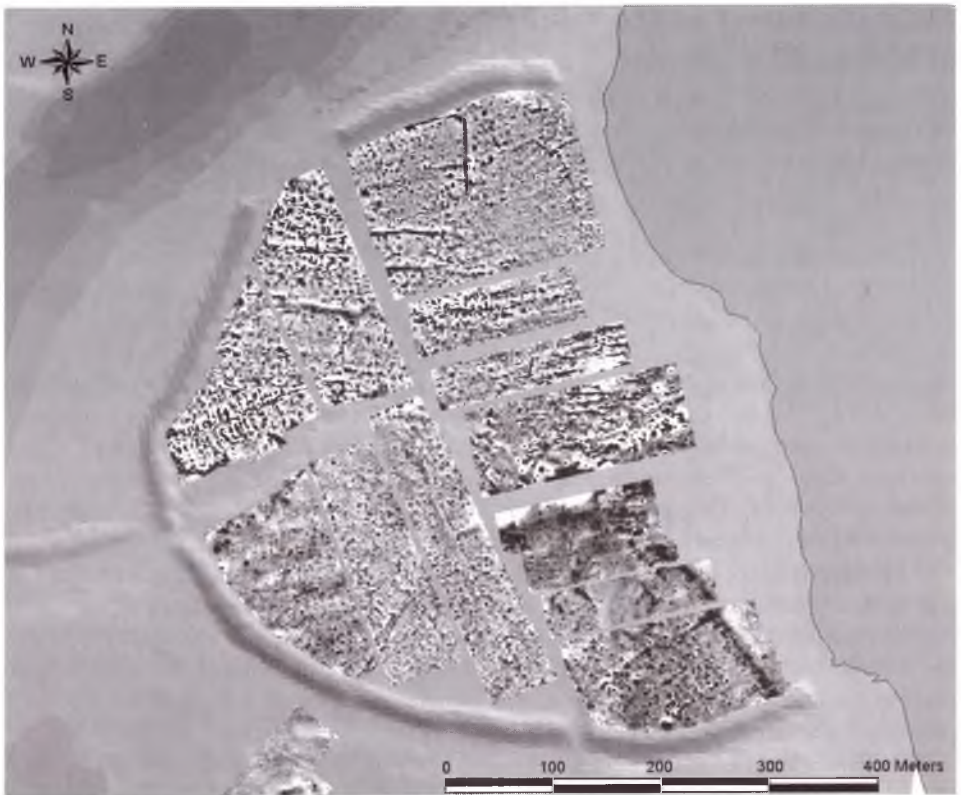
Fig. 1. Haithabu. Combined results of the magnetic survey by the teams from Munich and Vienna, measured with Cs-sensors.
