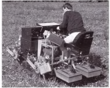
Fig. 1. Modified small caterpillar vehicle for simultaneous recording of GPR and resistivity data (spike wheels). Two antennas mounted with a distance of 50 cm at the end.
