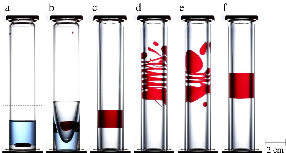
Figure S16. Formation and stretching of a cylindrical rim of an “intermediate” liquid (DMSO) between two immiscible oils. Details of liquids and container are the same as in Figures S14 and S15 , yet the total amount of DMSO (red) is decreased to 0.5 mL. a , Steady-state at 70 rpm – such a slow speed of rotation does not visibly affect the shape of layers, but keeps DMSO in the center. b , at 750 rpm, DMSO finds its place around paraboloid interface of decane and air, but does not form a fully closed ring. c , at 3000 rpm both layers of oils are stretched along entire length of the tube, but for the layer of DMSO, due to its small volume, adapting such a configuration would require thickness below 45 \mu\text{m} , much lower than its capillary length. Instead, DMSO forms a cylindrical rim, with average thickness 0.49 mm. As a result of increasing rotational speed – accompanied by transient states d , and e , – to 4500 rpm, the rim changes position and stretches further, so that its thickness decreases to 0.33 mm in snapshot f . Note that ratio of thicknesses of this layer in stationary states ( c ) and ( f ), 0.49/0.33, as well as the ratio of its vertical height (from which the thicknesses were calculated) is almost equal to the ratio of rotational speeds, 1.5 – in accordance with the model described in Section S4.2 . In contrast to the rims in Figure S15f , vertical position of rims in ( c ) and ( f ) are not fixed with respect to the ends of the tube. Depending on the history of \omega vs. time, the rims may form at different vertical positions and even for constant \omega they may slowly migrate along the tube – although it is not clear whether they do so to minimize total surface energy, or in response to random external factors, including vibrations or thermal drifts.
