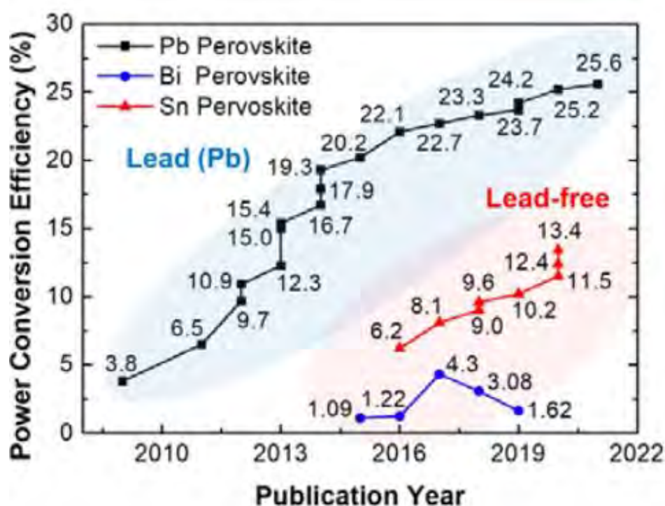
Fig. 1.5: Progress in PCE of Pb-based and Pb-free perovskite solar cells since 2009 (adapted from 28 ).
