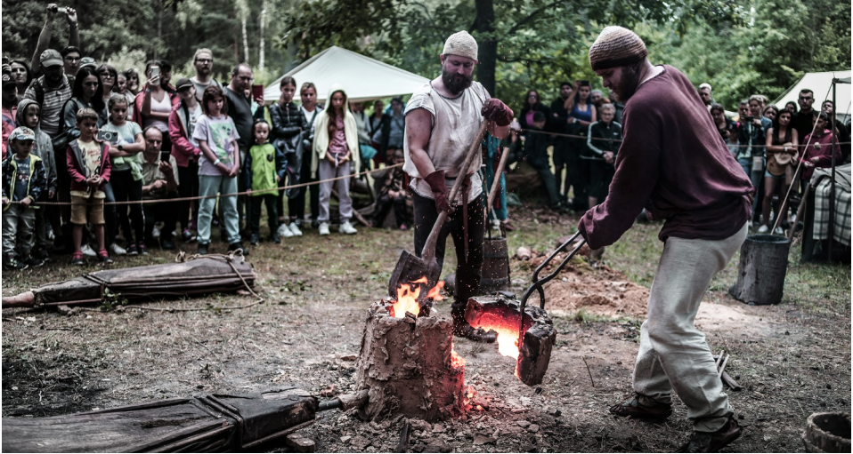
Fig. 10. The dismantling of a slag-pit furnace in order to obtain iron in the course of an experiment carried out during the “Ostrowiec Festival of Prehistoric and Ancient Culture”. Photo: K. Dziewięcki.
