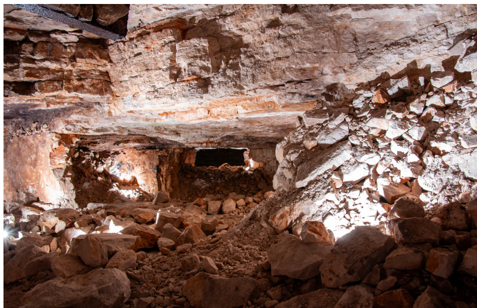
Fig. 1. View of the excavation of pillar-chamber mines seen from the tourist route. Photo: K. Cybulska.
