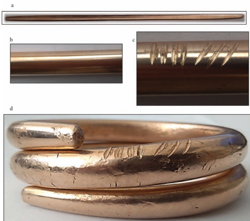
Fig. 15. CuSn3 alloy bracelet: a – casting of the bar, b – surface of the bar after polishing, c – the shape and arrangement of the ornament, d – a bracelet wrapped from casting bar. Prepared by B. Pisarek
