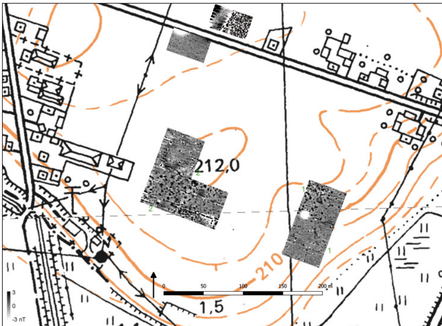
Fig. 20. Opatkowice, Proszowice district, site 3. Magnetic map in greyscale imposed on a topographic map. The green numbers indicate anomalies discussed in the text. Drawn by M. Podsiadło, M. M. Przybyła
