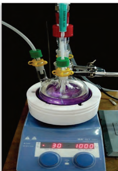
Figure 7. Batch reactor used for sorption experiments and catalytic hydrodechlorination of chloroorganic contaminants in water.
