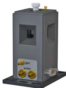
Figure 3.12: A photograph of the LUMA40; there are four rectangles optical ports, two connectors for the water flow, one connector for dry gas inlet and an electrical communication port at the bottom right.
