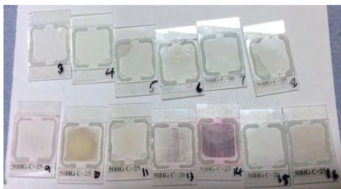
Figure B.3: A photograph of R6G samples after 12 kV/cm DC field for 5 minutes
