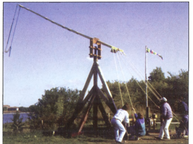
Fig. 15. Traction trebuchet. Replica in the Medieval Centre, Nykøbing Falster. Photo: Middelaldercentret, Nykøbing Falster, Denmark.
