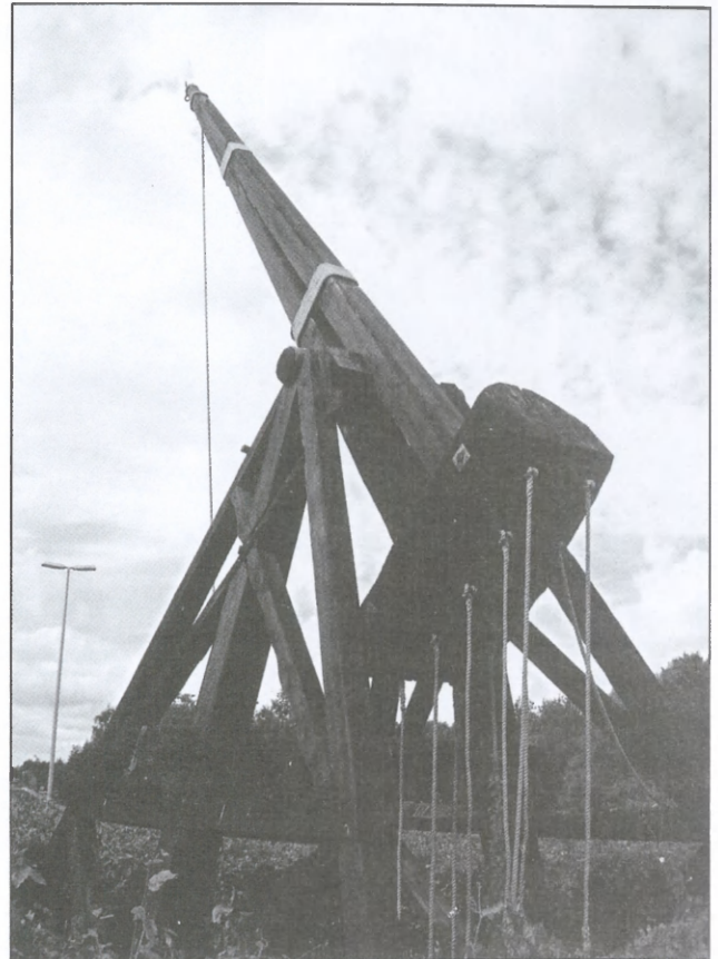
Fig. 17. Hybrid trebuchet. Replica in the Medieval Centre, Nykøbing Falster. Photo: S. Ekdahl.
