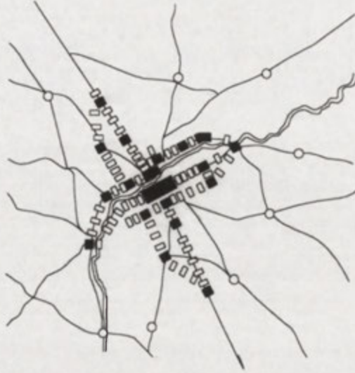
Figure 3. Concept of 'dynamical belts' in the Chmielewski's and Syrkus model of 1934. This model is a prototype of the city-region, black rectangles—units of potential development, according to Malisz (1966)
