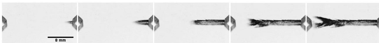
Fig. 1. Crack evolution in V-notched samples with thickness 9.7 mm (recording angle -15^\circ ).
